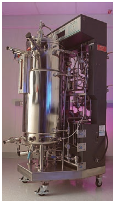
Engineers grow modified microbes in bioreactors such as this one, and harvest their products.
