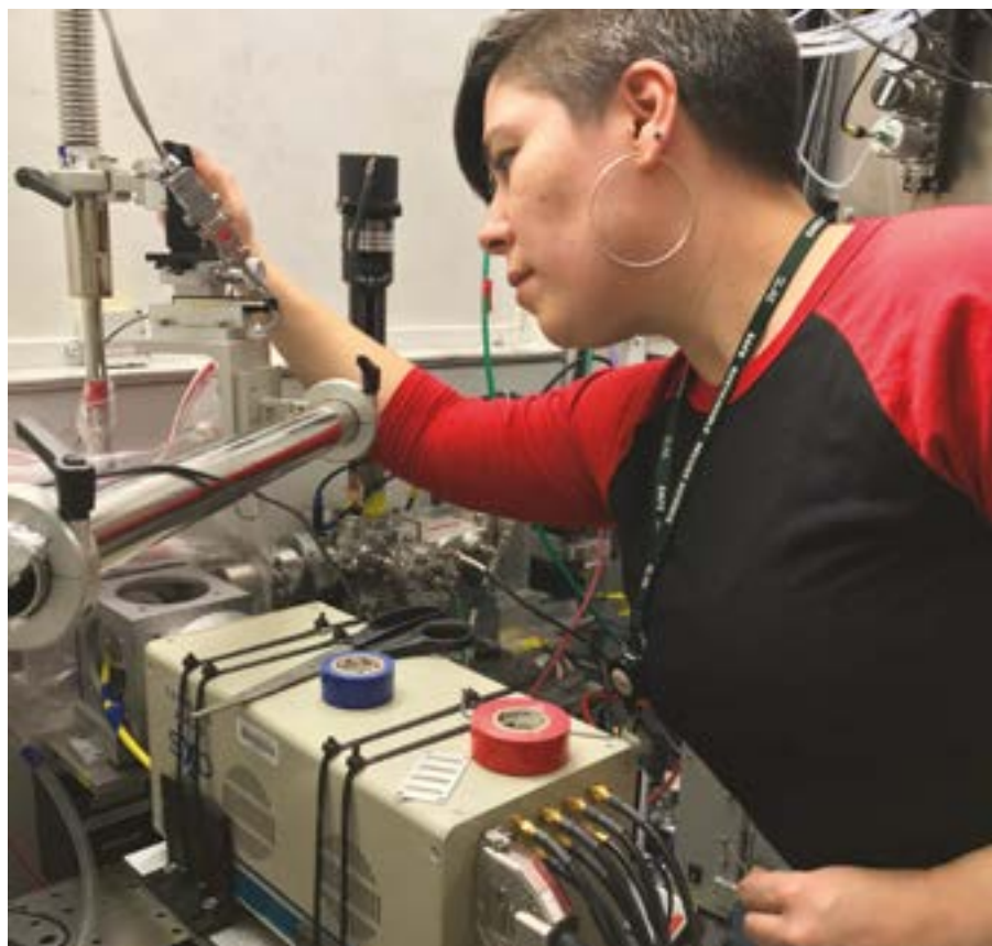
Kelly Chacón prepares a protein sample to be analyzed by X-ray absorption spectroscopy at Beamline 4-3, a side station at the Stanford Synchrotron Radiation Lightsource in Menlo Park, California. She is using tender x-rays to probe sulfur oxidation state in sulfur homeostasis proteins.
