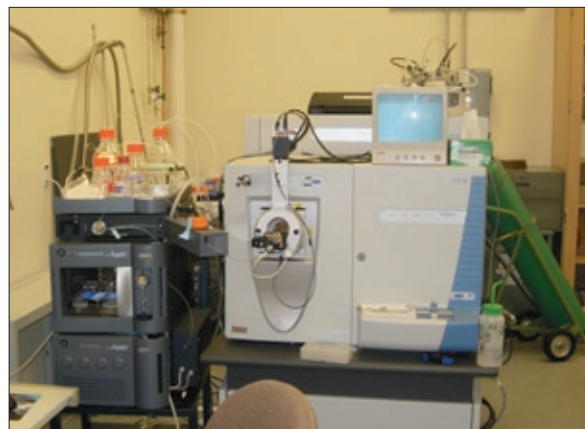
An Orbitrap mass spectrometer with electron transfer dissociation (ETD) connected to a high pressure liquid chromatography system from Waters, one of UCSF’s new machines that will tackle post-translational modifications in histones and chromatin.
